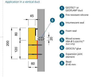
In the case of a GEOFLAM  $^{\ensuremath{\otimes}}$  duct, use fiber reinforced gypsum instead of wood screws.
