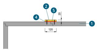
Cover strips used to reinforce large vertical ducts
