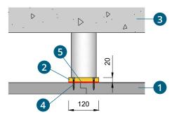
Cover strips used to reinforce the upper board of horizontal ducts
