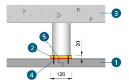
*Cover strips used to reinforce the upper board of horizontal ducts*
