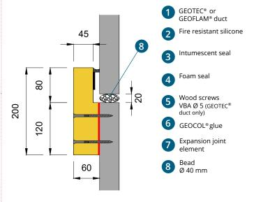
In the case of a GEOFLAM  $^{\ensuremath{\otimes}}$  duct, use fiber reinforced gypsum instead of wood screws.
