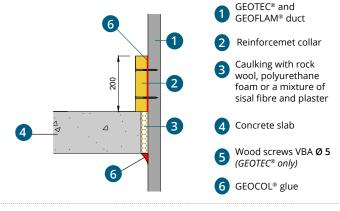
Reinforcement collar used as internal reinforcement for GEOTEC® horizontal ducts
