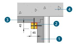
Batten used in a vertical duct when abutting the wall
