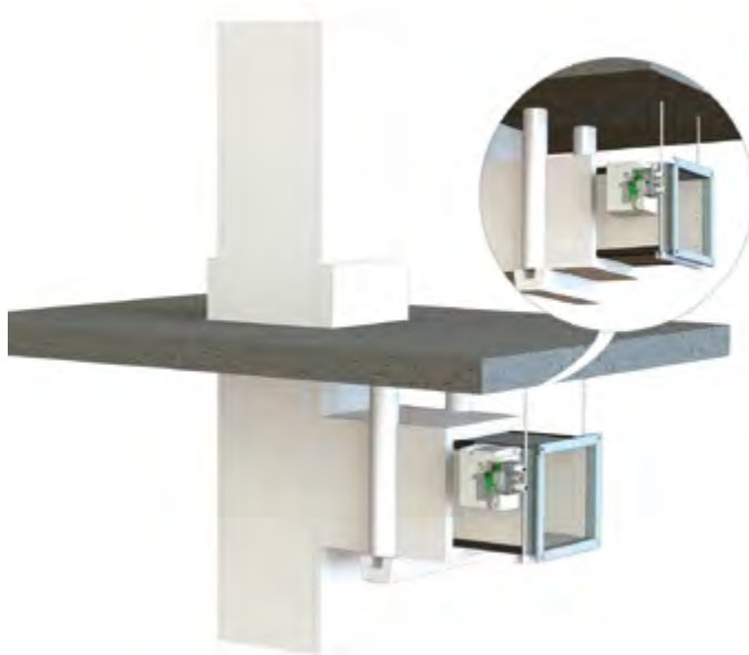
installation of a fire damper
