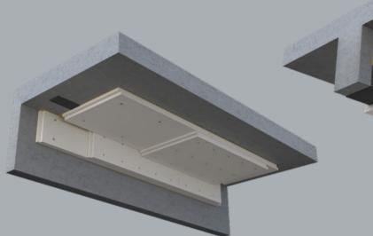
In this configuration, a GEOCOL<sup>®</sup> adhesive is applied to the periphery of the carbon reinforcement.
