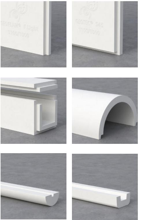
**GEOTEC® and GEOFLAM® fire-resistant boards** enable you to create horizontal and vertical ventilation and smoke extraction ducts rated EI 60 to EI 240; build 2-hour fire protection enclosures; protect bonded carbon reinforcement; and protect cable trays.
